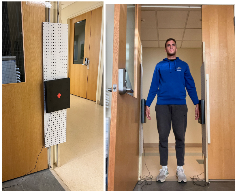
Figure 1. (A) Wooden stands with a force plate attached enabled recording of force generated during the experiment. (B) Subjects pressed against force plates with the back (dorsal) surface of the hands.
