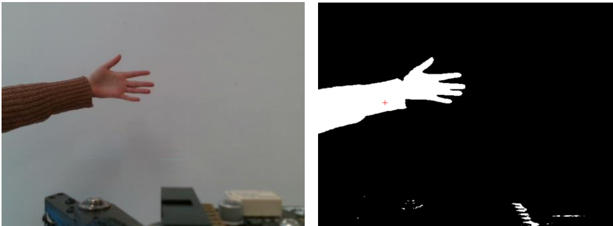
Figure 11. Image of hand and center of mass that passed test 1. The image on the left is the RGB image of the hand. The image of the right is the segmented image of the hand with a red 'x' marking the calculated center of mass. In this image, the forearm was also considered part of the hand. In this case, the center of mass was calculated to be on the person's forearm instead of being on the actual hand.
