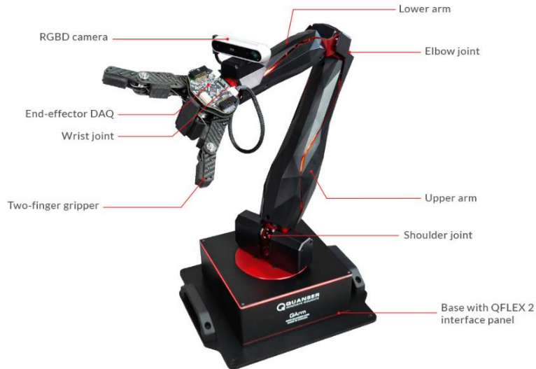
Figure 1. Labeled image of the Quanser QArm
