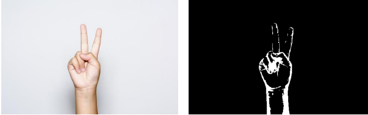
Figure 9. Image of unsuccessfully detected hand. The image on the left is the RGB image of the hand. The image on the right is the segmented image of the hand. In this case, only the edges of the hand were detected, and therefore only the edges of the hand were segmented properly. This caused a hand to not be detected since less than 10% of the image was considered a hand.
