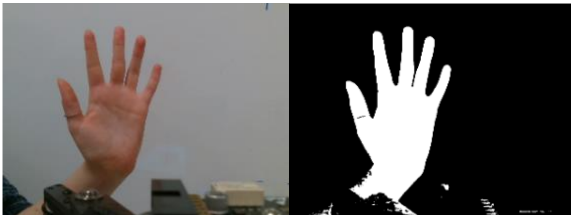
Figure 4. RGB image of hand compared to the segmented image. The image on the left is the RGB image of the hand. The image on the right is the black and white segmented image of the same hand. Everywhere in the image where a hand is detected is white, the rest is black.
